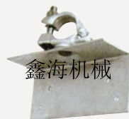
XIN-A038 防滑杠焊接直角扣件 Coupler with Welded Plate Φ48.3mm 2.10Kg
